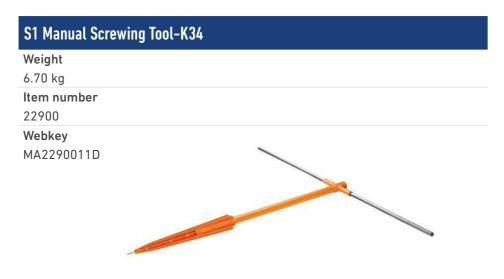
To drive KSF K34 x 550 ground screws into soft to medium soil types manually. As for pinpoint accuracy and easy installation, we recommend pre-drilling with a hammer drill or rotary hammer. The drill bit should be at least 40 mm in diameter and approximately 800 mm long. A little water can also be poured into the predrilled borehole before inserting the screw for optimal lubrication.
