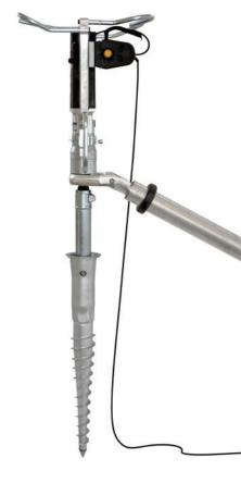
To drive small to medium-sized ground screws into the soil up to Class III manually. As for pinpoint accuracy and easy installation, we recommend predrilling with a hammer drill or rotary hammer. The drill bit should be at least 40 mm in diameter and approximately 800 mm long. A little water can also be poured into the borehole after drilling for optimal lubrication.
