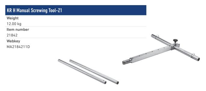
To drive small to medium-sized ground screws into the soil up to Class III manually. As for pinpoint accuracy and easy installation, we recommend predrilling with a hammer drill or rotary hammer. The drill bit should be at least 40 mm in diameter and approximately 800 mm long. A little water can also be poured into the predrilled borehole before inserting the screw for optimal lubrication.
