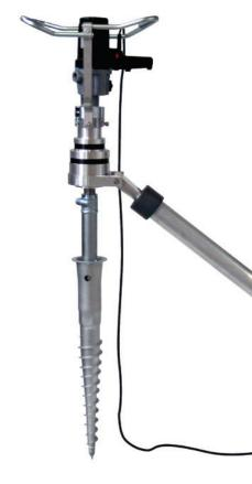
To drive small to medium-sized ground screws into the soil up to Class III manually. As for pinpoint accuracy and easy installation, we recommend predrilling with a hammer drill or rotary hammer. The drill bit should be at least 40 mm in diameter and approximately 800 mm long. A little water can also be poured into the borehole after drilling for optimal lubrication.
